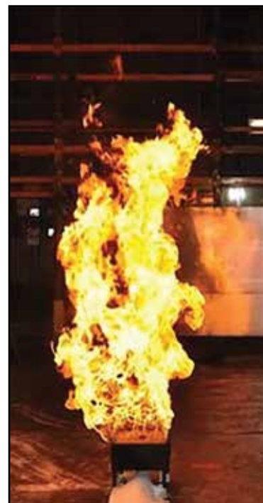
Figure 1 Flames from a free-burning fire, away from walls or ceiling. A 0.3x0.3 m (1x1 ft) propane burner is producing 500 kW/m 2 of HRR per unit area (Photo: Oskar Lind and Per Troedson)
