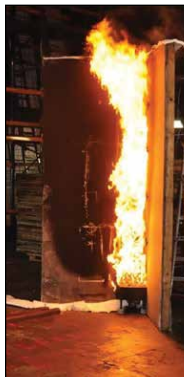
Figure 2 Flames in a corner, from a burner providing 5555 kW/m 2 (Photo: Oskar Lind and Per Troedson)
