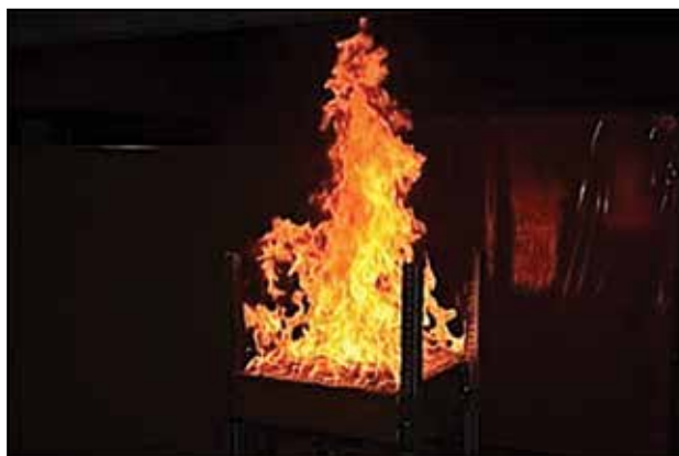
Figure 3 Flames from a burner providing 317 kW from a 0.6x0.6 m (2x2 ft) face area, which is equivalent to 880 kW/m 2 . (Photo: Jason Huczek; copyright 2016 Interscience Communications Ltd)
